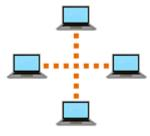
**Wide Area Network (WAN)**: A WAN typically consists of two or more LANs. The computers are farther apart and are linked by telephone lines, dedicated telephone lines, or radio waves. The **Internet** is the largest Wide Area Network (WAN) in existence.
